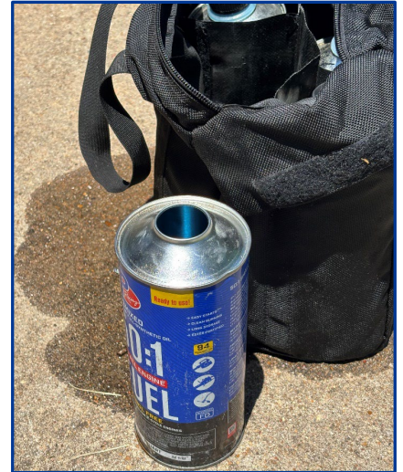
The premixed fuel can, after its plastic spout had popped off, beside the fuel bag that held it.
